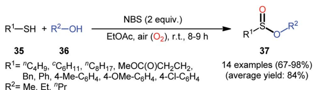
Scheme 17 NBS-mediated oxidative esterification of thiols 35 with alcohols 36 .
