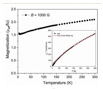
Fig. 1 Magnetic properties of Na[o-<sup>57</sup>FESAN] powder sample: temperature dependence of the magnetization under a magnetic field of 0.1 T. Inset: temperature dependence of the inverse of the magnetic susceptibility. The solid red line is the fit to the Curie-Weiss law of the experimental data (solid square symbols).
