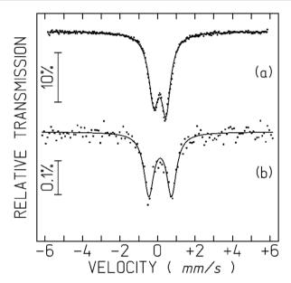
Fig. 3 Mössbauer spectra of Na[o-57FESAN] (a), and the U87 cells incubated with Na[o-57FESAN] (b) taken at 80 K in the solid state. The lines over the experimental points are fitted quadrupole doublets. The estimated parameters are collected in Table 1.
