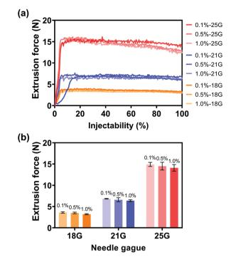
Fig. 10 (a) Extrusion force curves and (b) average extrusion force of alg-Au NPs synthesized in different alginate concentrations through different needles
