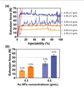
Fig. 4 (a) Extrusion force curves and (b) average extrusion forces of different concentrations of Au NPs (prepared by ethanol reduction in ethanol/water mixture without stabilizing molecules) of the injection medium with sodium alginate concentration. Needle gauge: 18 G.
