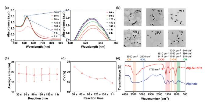
Fig. 9 (a) UV-Vis spectrum, (b) TEM, (c) average sizes, and (d) CV of alg-Au NPs synthesized with 0.5% w/v alginate aqueous solutions. (e) FTIR of alg-Au NPs and alginate. The scale bar is 50 nm.
