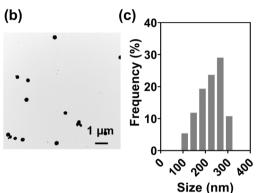
Fig. 2 (a) UV-Vis spectrum, (b) TEM image, and (c) size distribution (taken from TEM image) of Au NPs prepared via an ethanol reduction method in pure water/ethanol mixed solvent without any stabilizing molecules.
