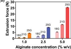
Fig. 3 (a) Extrusion force curves and (b) average extrusion forces of injection media with different concentrations of aqueous solutions of sodium alginate when passing through different gauge needles.
