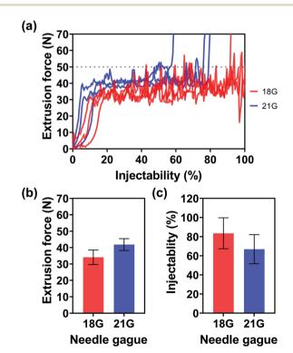
Fig. 5 (a) Extrusion force curves, (b) average extrusion force, and (c) injectability (ratio of injected volume/total volume with extraction force of 50 N) through different needle gauges. Injection medium: sodium alginate with a concentration of 2.5% w/v; Au NP concentration: 0.5 g mL<sup>-1</sup>
