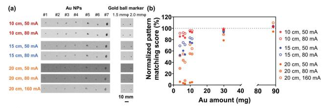
Fig. 6 (a) X-Ray visualization image of gold ball markers and samples with different amounts of Au NPs under different acrylic resin thicknesses and tube currents. (b) Relationship between normalized pattern matching scores and different gold amounts.
