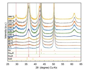
Fig. 5 In situ heating XRD patterns of 1-hexanoic acid-stabilised copper nanoparticles. The sample was heated under air.
