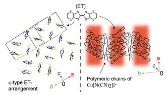
Fig. 1 Crystal structure of 1. Blue, violet, yellow, orange, and green spheres represent C, N, S, Cu, and I atoms, respectively. The H atoms were omitted for clarity. Two-dimensional conduction pathways are highlighted in red
