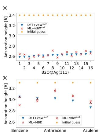
**Fig. 6** (a) Adsorption heights of B2O molecules on Ag(111). (b) Adsorption heights of benzene, <sup>82</sup> naphthalene, <sup>83</sup> anthracene, <sup>84</sup> pentacene, <sup>85</sup> and azulene, <sup>85</sup> computed with ML+vdW<sup>surf</sup> and compared to DFT+vdW<sup>surf</sup>. The same adsorption sites as mentioned in the cited references (Table 1) are used.
