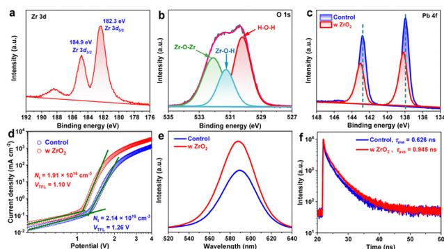
**Fig. 2** (a) Zr 3d and (b) O 1s regions of the XPS spectrum of the ZrO<sub>2</sub>-capped perovskite film. (c) Pb 4f XPS spectra of perovskite films with and without a ZrO<sub>2</sub> layer. (d) Dark *J*-*V* curves of electron-only devices for SCLC analysis. (e) Steady PL spectra and (f) TRPL decay curves of the indicated perovskite films.
