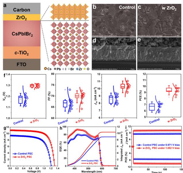
**Fig. 1** (a) Illustration of the structure of the ZrO<sub>2</sub>-capped device. (b and c) Top-view SEM images of perovskite films with and without the ZrO<sub>2</sub> capping layer. (d and e) Cross-sectional SEM images of the PSCs. (f) Statistical photovoltaic parameters of control and optimal PSCs. (g) *J*-*V* curves, (h) EQE spectra and (i) steady power output curves of control and optimal PSCs.
