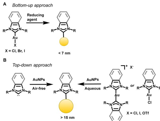
Fig. 7 Synthetic approaches to append NHCs to AuNPs. Both bottom-up and top-down approaches have proven successful.
