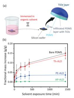
Fig. 3 (a) Measurement of organic solvent resistance performance of the samples (made with biorender.com), (b) fractional mass increase of bare and ALD-treated PDMS, cured at 200 °C. Error bars of bare PDMS were calculated as the standard deviation of 20 samples per time point, while error bars of the ALD treated PDMS were based on 3 samples.
