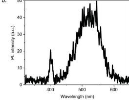
Fig. 3 Photophysical properties of  $[Ag_2(1,3-BDT)]_n$ : (a) temperature-dependent solid state emission spectra ( $\lambda_{ex} = 410 \text{ nm}$ ) and (b) second harmonic generation response with incident beam at  $\lambda_{ex}$  = 800 nm and RT.
