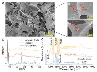
Fig. 2 Characterization of the hybrid aerogel. (a and b) SEM images of the inner structure of the hybrid aerogel. (c) The XRD patterns and (d) FTIR spectra of amyloid fibrils, hybrid aerogels, and UiO-66-NH<sub>2</sub>.
