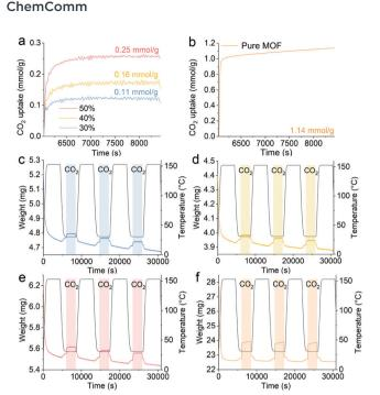
Fig. 3  $CO_2$  capture performance of (a) hybrid aerogels with different MOF loadings and (b) pure MOF, (c-f) weight changes for three consecutive cycles of  $CO_2$  sorption-desorption of hybrid aerogels with 30%, 40%, 50% MOF and pure MOF, respectively.
