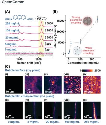
Fig. 2 (A) SERS spectra of MB added to the Plasmonic bubble film with varying nanocube concentrations. (B) Signal intensity of the 1633 cm<sup>-1</sup> peak. (C) Hyperspectral SERS map for increasing Ag concentrations (mg mL<sup>-1</sup>): (i and ii) 5, (iii and iv) 20, (v and vi) 100 and (vii and viii) 250.
