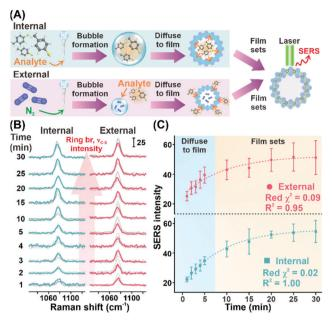
Fig. 4 (A) Two different modes of gas sensing. (B) Time-dependent SERS spectra of MBT show the increase in the intensity of the 1077 cm<sup>-1</sup> peak. (C) Comparing the SERS signal intensity of MBT using two different modes of analyte sensing
