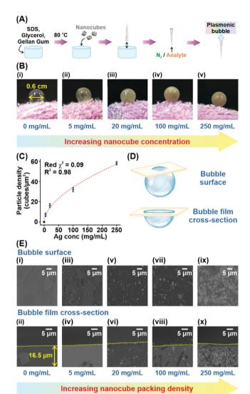
Fig. 1 (A) Formation of a Plasmonic bubble. (B) Plasmonic bubble with varying Ag nanocube concentrations (mg mL<sup>-1</sup>): (i) 0, (ii) 5, (iii) 20, (iv) 100 and (v) 250. (C) Relationship between nanocube concentration and packing density in the bubble film. (D) The bubble surface and bubble film cross-section. (E) SEM images for Ag nanocube concentrations (mg mL $^{-1}$ ): (i and ii) 5, (iii and iv) 20, (v and vi) 100 and (vii and viii) 250
