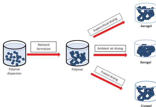
Fig. 2 Schematic routes to fabricate polymer gel network and dried gels, case of PEDOT:PSS. The polymer chains are represented by the dark blue beads while the solvent (water) is in light blue.
