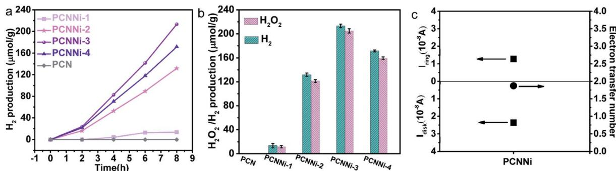
Fig. 4 (a) Photocatalytic hydrogen generation from pure water under visible light ( $\lambda > 420$  nm), (b) photocatalytic overall water splitting into hydrogen and hydrogen peroxide without any sacrificial reagent under visible light ( $\lambda > 420$  nm) with activity marked by the error bar, (c) the measured Pt disk current and Pt exchange current and corresponding electron transfer number.
