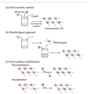
Fig. 1 General synthesis methods for heterometallic coordination polymers: (a) self-assembly method, (b) metalloligand approach, and (c) post-synthesis modification.
