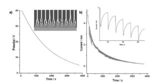
Fig. 10 (a) Potential-time and (b) current-time transients profiles recorded in non-steady-state anodization. Inset in (a) is a schematic illustration of the tree-like branched pores. Inset in b is the magnification of the current curve for a clear view of its tooth-like profile. Reprinted with permission from ref. 209. Copyright © 2007, The Royal Society of
