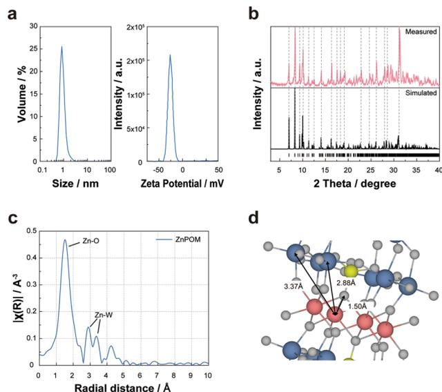
**Fig. 1** Characterization of ZnPOM. (a) Dynamic light scattering (left) and zeta potential (right) analyses of ZnPOM. (b) Simulated and measured XRD patterns of ZnPOM. (c) EXAFS analysis showing the distance between Zn and its nearest neighbouring elements in ZnPOM. (d) A graphical illustration showing the molecular structure of ZnPOM and coordination environment of  $\text{Zn}^{2+}$  ions in ZnPOM.
