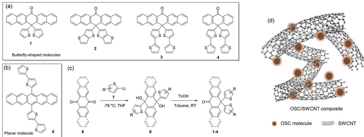
**Scheme 1** (a) Molecular structures of the studied butterfly-shaped OSCs **1–4**. (b) Molecular structure of the studied planar molecules **5**. (c) Synthesis of the butterfly-shaped OSCs **1–4**. (d) Illustration of the OSC/SWCNT composites.
