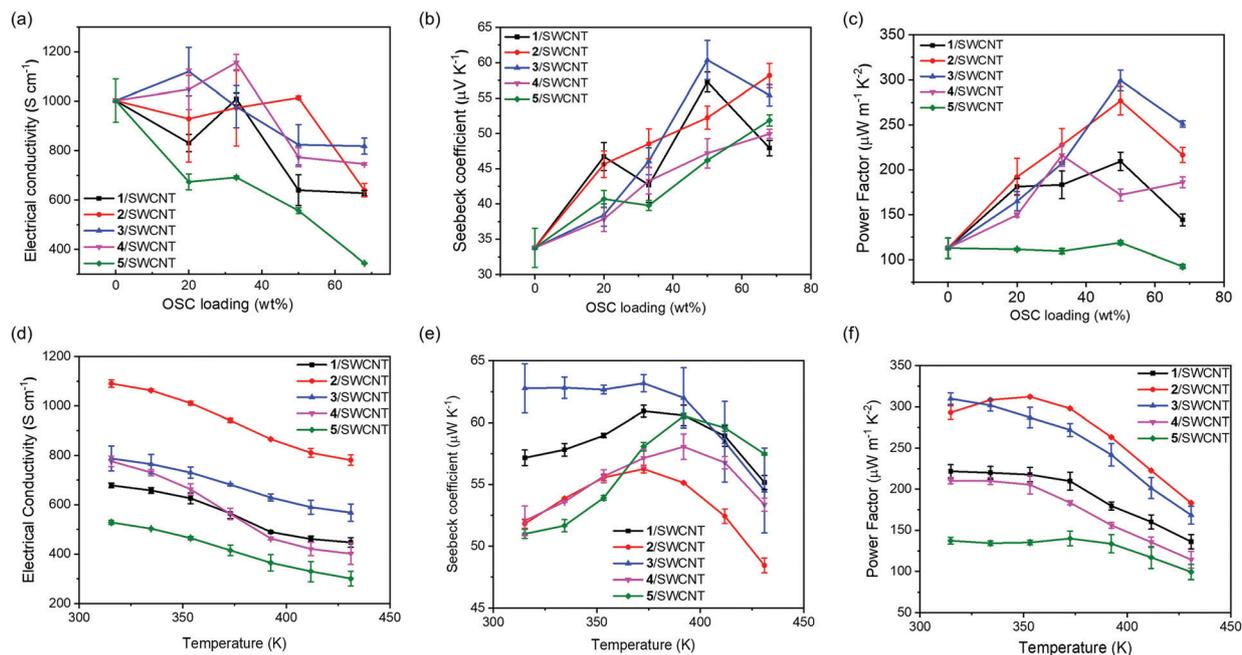
Fig. 3 The  $\sigma$  (a),  $S$  (b), PF (c) values of OSC/SWCNT composite films at different OSC loadings. The temperature dependency of the  $S$  (d),  $\sigma$  (e), PF (f) values of OSCs/SWCNT composite films at OSC loading of 50%.
