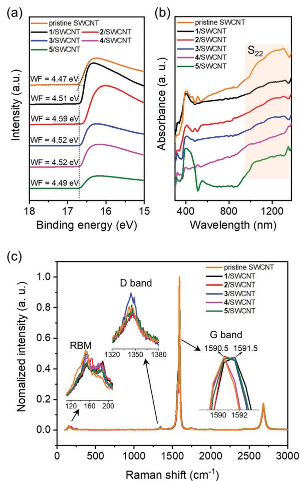
Fig. 5 Photophysical characterization of pristine SWCNT and OSCs/SWCNT composite films with OSC loading of 50%: (a) UPS spectra, (b) UV-vis-NIR spectra, and (c) Raman spectra.
