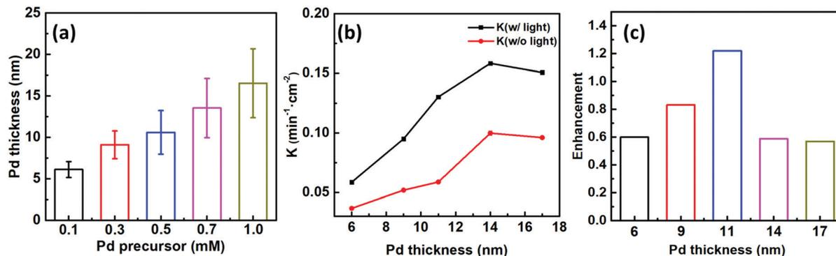
Fig. 3 The effect of the Pd thickness on the plasmon-enhanced catalytic property of the Janus plasmene nanosheets. (a) Thickness change of Pd on Au NC nanosheets with increasing concentration of the Pd precursor. (b) Catalytic rate (normalized to the geometric surface area of the plasmene) of Janus plasmene nanosheets with different Pd thicknesses w/light (black curve) and w/o light (red curve) and (c) their corresponding plasmon enhancement.
