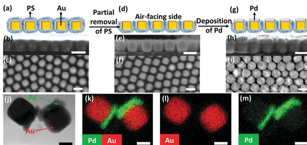
**Fig. 1** Fabrication of Janus plasmene nanosheets. (a, d, and g) Scheme of fabricating Janus plasmene nanosheets. Cross-section SEM image of (b) PS-capped, (e) one-side exposed and (h) Janus plasmene nanosheets on a Si wafer and (c, f, and i) their corresponding top-view SEM images. (j) Dark-field TEM images of individual Janus NPs and (k–m) corresponding EDX elemental mapping images (red: Au; green: Pd). (Scale bar: 50 nm for SEM, 20 nm for TEM.)
