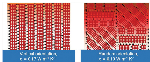
Fig. 12 Schematic illustrations of vertically and randomly oriented \text{BA}_2\text{MA}_3\text{Pb}_4\text{I}_{13} crystal orientations that lead to different thermal conductivities. Reprinted with permission from ref. 32. Copyright (2020) American Chemical Society.
