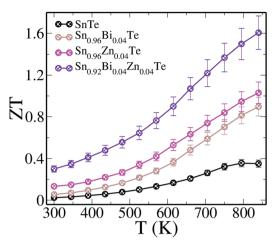
Fig. 5 ZT of SnTe and doped samples as a function of temperature. The ZT measurement uncertainty is about 10% (error bar).
