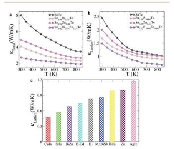
Fig. 4 (a) Total thermal conductivity; (b) lattice thermal conductivity of SnTe and doped samples as a function of temperature; (c) comparison of lattice thermal conductivity of Sn $_{0.92}$ Bi $_{0.04}$ Zn $_{0.04}$ Te with the state of the art SnTe based materials.  $^{6-9,17,19,22,23}$
