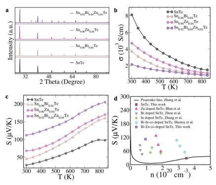
Fig. 3 (a) XRD pattern (\* indicates peaks due to the Zn precipitate); (b) electrical conductivity; (c) Seebeck coefficient of SnTe and doped samples as a function of temperature; (d) Seebeck coefficient values of SnTe and Bi-Zn co-doped SnTe at 300 K as a function of carrier concentration 'n' in comparison with the Pisarenko line and earlier reports.  $^{7-9,31}$
