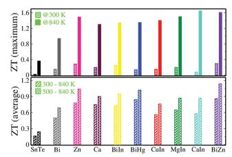
**Fig. 6** Comparison of *ZT* at 300 K and 840 K (upper panel);  $ZT_{average}$  of SnTe and Sn<sub>0.92</sub>Bi<sub>0.04</sub>Zn<sub>0.04</sub>Te (lower panel) with the reported high performing SnTe based materials.<sup>7–9,11,14,18–20</sup>
