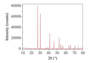
Fig. 1 X-ray diffraction pattern of  $Ba_3VWO_{8.5}$  which can be indexed by the R3m H space group.
