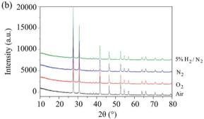
Fig. 2 (a) XRD patterns of  $Ba_3VWO_{8.5}$  recorded after a 24 hour anneal in air at selected temperatures. (b) XRD patterns of  $Ba_3VWO_{8.5}$  recorded after 24 hours annealing at 900 °C under different flowing gases (air,  $O_2$ ,  $N_2$ , 5%  $H_2/N_2$ ).
