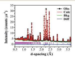
Fig. 5 Fitted neutron diffraction histogram for  $Ba_3VWO_{8.5}$  at ambient temperature. The TOF neutron diffraction data from the  $90^\circ$  bank detector of the Polaris diffractometer is shown. Black dots indicate the observed data, the red line the Rietveld fit, the blue line indicates the difference between the observed and the calculated patterns, the green line the background function, and the pink vertical bars the reflection positions.
