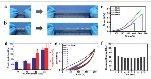
Fig. 2 The mechanical properties of the gelatin organohydrogels. Photographs showing (a) stretching and (b) curly stretching of the gelatin organohydrogels. (c) Tensile curves and (d) the corresponding elastic modulus and toughness of the gelatin organohydrogels soaked in different Na<sub>3</sub>Cit concentration solutions. (e) Ten successive cyclic tensile loading–unloading curves and (f) the dissipated energy of the gelatin organohydrogel (20 wt% Na<sub>3</sub>Cit).
