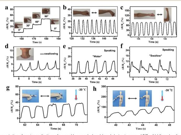
Fig. 6 Demonstration of sensing applications of a wearable organohydrogel-based electronic sensor.  $\Delta R/R_0$  of (a) finger bending at various angles, (b) elbow rotation and (c) wrist bending. Detection of subtle motions of (d) swallowing and pronouncing different words: (e) "water" and (f) "swallow". The wearable electronic sensor attached to (g) a prosthetic finger for monitoring finger bending and (h) human model for detecting elbow rotation at -30 °C.
