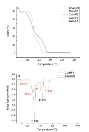
$\begin{tabular}{ll} Fig. 6 & (a) TGA curves of original sawdust and CWNF films and (b) DTG curve of the CWNF4 film with original sawdust. \\ \end{tabular}$
