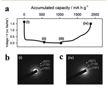
Fig. 17 (a) First galvanostatic charge and discharge profiles of the Sn<sub>4</sub>P<sub>3</sub> electrode obtained without an FEC additive. The different points indicate (i) pristine, (ii) 0.07 V, (iii) 0 V and (iv) 1.5 V. (b, c) Electron diffraction (ED) patterns at the points (i) and (iv) in (a), respectively. Reproduced with permission.<sup>77</sup> Copyright 2014, WILEY-VCH.
