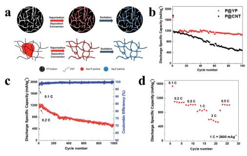
Fig. 8 (a) Schematics of the preparation and sodiation of P@YP and P@CNT composites. (b) Cycling performances of P@YP and P@CNT composites within 100 cycles. (c) Long term cycling performance of the P@YP composite. (d) Rate performance of the P@YP composite at C-rates between 0.1C and 3C ( $1C = 2600 \text{ mA g}^{-1}$ ). Reproduced with permission: (a) Reproduced to Copyright 2017, Elsevier Ltd.
