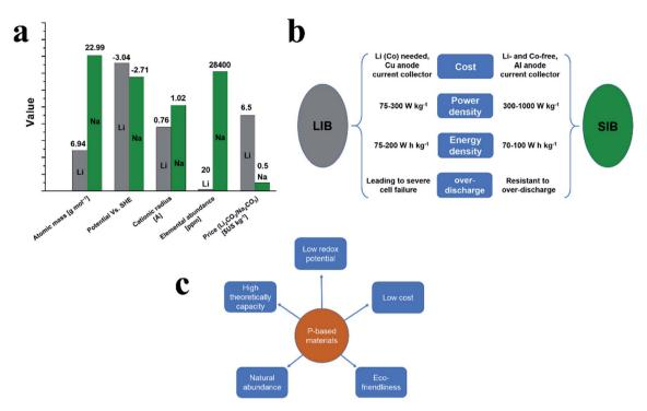
Fig. 1 (a) Major property differences between lithium and sodium; (b) main differences between lithium-ion batteries (LIBs) and sodium-ion batteries (SIBs); (c) main advantages of phosphorus/phosphides as anode materials for SIBs.
