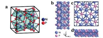
Fig. 23 (a) Crystal structure of cubic Ni<sub>3</sub>P. Reproduced with permission. 199 Copyright 2014, The Royal Society of Chemistry. (b) Crystal structure of hexagonal Ni<sub>2</sub>P: four unit cells stacked on top of one another, with a single unit cell outlined. (c) Top-down view of the Ni<sub>2</sub>P (001) surface. (d) A two-dimensional slice of Ni<sub>2</sub>P, showing the (001) surface on top. Reproduced with permission.<sup>249</sup> Copyright 2013, American Chemical Society
