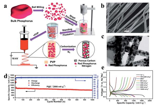
Fig. 5 (a) Schematic illustration of the preparation process for RP@C nanofibers. (b, c) SEM and TEM images of red P@C nanofibers. (d) Longterm cycling stability of the P@C electrode at a current density of 2000 mA g<sup>-1</sup>. (e) Charge/discharge profiles obtained at various rates of the P@C electrode in the voltage range of 0.01-2 V vs. Na<sup>+</sup>/Na. Reproduced with permission.<sup>127</sup> Copyright 2017, Elsevier B.V.
