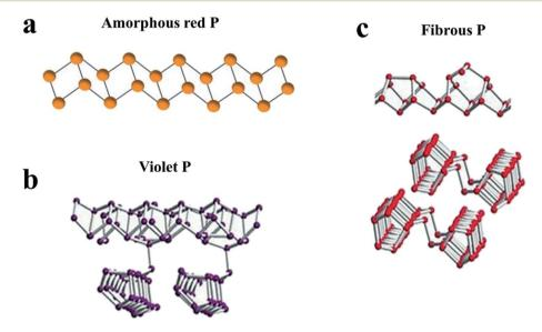
Fig. 2 Characteristic structural fragments of (a) amorphous RP; (b) violet P (Hittorf's P); (c) fibrous P. (a) Reproduced with permission. Copyright 2019, WILEY-VCH. (b, c) Reproduced with permission. Copyright 2017, Wiley-VCH.
