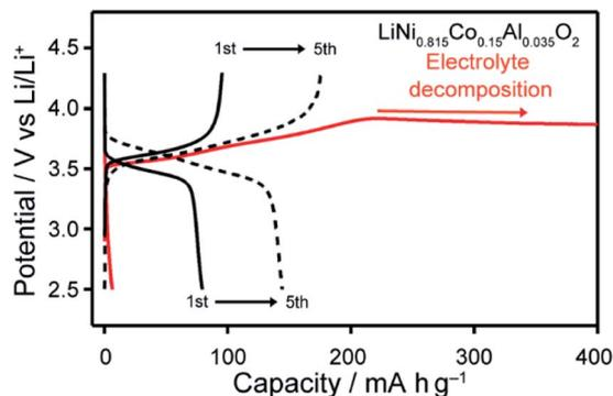
Fig. 9 Charge-discharge curves of Li half-cells composed of LC electrolytes of 1/LiTFSI (black) and 3/LiTFSI (red), and  $\text{LiNi}_{0.815}\text{Co}_{0.15}\text{Al}_{0.035}\text{O}_2$ , recorded at 80 °C.
