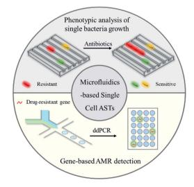
Fig. 1 Microfluidic technologies for rapid antibiotic susceptibility tests (ASTs) at the single-cell level, including both phenotypic analysis (microfluidic-based single bacterial culture) and gene-based antimicrobial resistance (AMR) detection (droplet digital analysis).
