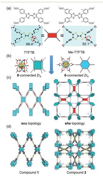
Fig. 1 Topologically guided steric tuning strategy for MOF design (a) TTFTB and Me-TTFTB linkers with different conformations. (b) 8connected and 6-connected Zr<sub>6</sub> clusters. (c) Targeted topologies formed by Zr<sub>6</sub> clusters and conformationally differing linkers. (d) Crystal structures of compounds 1 and 2. Color scheme: Zr, cyan; O, red; C, black; S, yellow.
