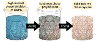
Fig. 6 Cartoon of the high internal phase emulsion templating route to prepare open porous macroporous foams.
