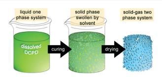
Fig. 7 Schematic preparation of aerogels.
