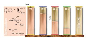
Fig. 4 Frontal polymerisation of pDCPD according to ref. 28
