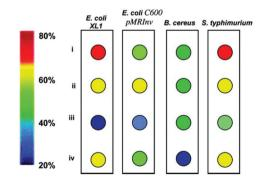
Fig. 13 Colorimetric bacterial fingerprinting. The color combination for each bacterium reflects the red chromatic shift (RCS) values recorded 7 h after the start of growth at a bacterial concentration of  $1\times10^9$  mL $^{-1}$ . The RCS color key is shown on the left. (i) DOPE/PDA (1:9 mole ratio); (ii) sphingomyelin/cholesterol/PDA (7:3:90); (iii) DMPC/PDA (1:9); and (iv) POPG/PDA (1:9). Reproduced from ref. 5 with permission from the American Chemical Society, copyright [2007].
