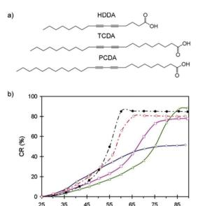
Fig. 6 (a) Chemical structure of DA monomers used to construct PDA/ZnO nanocomposites and (b) colorimetric response (CR) as a function of temperature. Symbols are for poly(PCDA) (○), poly(TCDA) (●), poly(PCDA)/ZnO (△), poly(TCDA)/ZnO (□), and poly(HDDA)/ZnO (◊) nanocomposites. Reproduced from ref. 36 with permission from Elsevier, copyright [2013].
