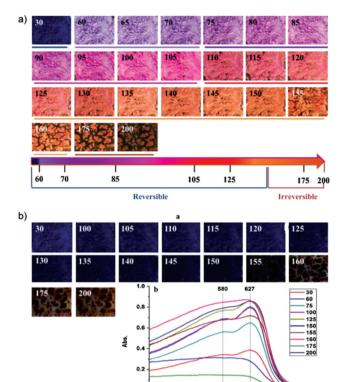
**Fig. 9** (a) Photographs of PDA-urea at temperatures ranging from 30 to 200 °C post-2 minutes equilibration. The color transition path with its reversibility upon heating is represented as the rainbow line. (b) Photographs of PDA-urea powders at room temperature after cooling. Reproduced from ref. 46 with permission from Elsevier, copyright [2017].
