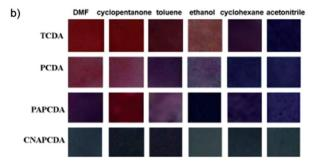
Fig. 7 (a) Colorimetric response and (b) photographs of PDAembedded polymer matrix films derived from TCDA, PCDA, PAPCDA, and CNAPCDA after exposure to organic solvents at room temperature. Reproduced from ref. 39 with permission from Elsevier, copyright [2010].
