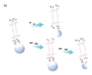
Fig. 18 (a) Photographs of aqueous suspensions of (a) pure poly (TCDA), (b) poly(PCDA)/ZnO (c) poly(TCDA)/ZnO, and (d) poly(HDDA)/ ZnO nanocomposites taken at different pH. (b) The ZnO dissociation model and color change mechanism of PDA/ZnO nanocomposites at low and high pH. Reproduced from ref. 61 with permission from Elsevier, copyright [2014].
