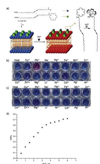
**Fig. 11** (a) The synthesis and binding mechanism of poly-PDA-L with Pb<sup>2+</sup>. PCDA-L and PCDA was mixed at 3:7 molar ratio. Digital images of the colorimetric responses of (b) poly-PDA-L and (c) pure PDA vesicles towards various metal ions (10  $\mu$ M) in HEPES buffer. (d) Colorimetric response (CR%) of poly-PDA-L at different Pb<sup>2+</sup> concentrations in HEPES buffer. Reproduced from ref. 48 with permission from Elsevier, copyright [2015].
