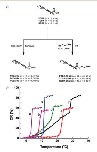
Fig. 10 (a) Schematic diagram of the preparation of diacetylene monomers to produce low temperature thermochromic PDA nanosensors. (b) Colorimetric response (CR) plot as a function of temperature of PDAs functionalized with ester moieties; (a) HCDA-EGME, (b) HCDA-Me, (c) TCDA-EGME, (d) TCDA-Me, (e) PCDA-EGME, (f) PCDA-Me, Reproduced from ref. 47 with permission from the American Chemical Society, copyright [2016].
