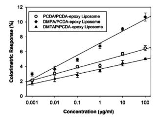
Fig. 15 Colorimetric response of PDA-phospholipid liposomes as a function of concentration of BVDV antibody. Reproduced from ref. 52 with permission from the American Chemical Society, copyright [2012].
