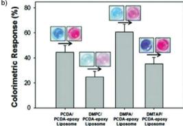
Fig. 14 (a) Transmission electron microscopy images of the different PDA-phospholipid liposomes. (b) Colorimetric response of PDA-phospholipid liposomes after 254 nm UV polymerization for a series of time periods and heating at 70 °C. Reproduced from ref. 52 with permission from the American Chemical Society, copyright [2012].
