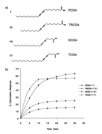
Fig. 5 (a) Chemical structure of 10,12-pentacosadiynoic acid (PCDA), 10,12-tricosadiynoic acid (TRCDA), 5,7-docosaciynoic acid (DCDA), and 5,7-tetracosadiynoic acid (TCDA). (b) Thermochromic colorimetric response of PDA vesicles composed of the different DA monomers after incubation at 50 °C as a function of time. Reproduced from ref. 30 with permission from the American Chemical Society, copyright [1998].
