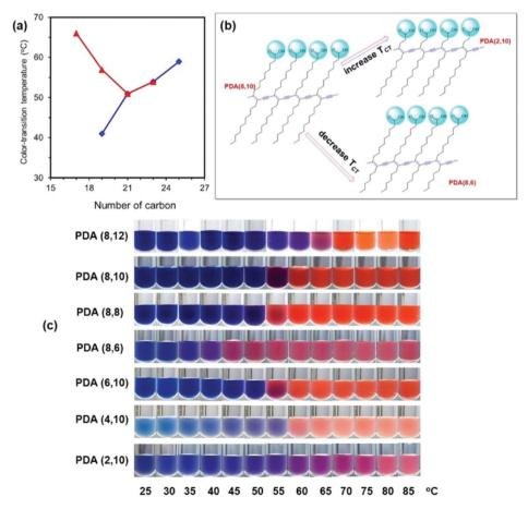
Fig. 8 (a) Plots of color transition temperature ( $T_{CT}$ ) versus number of carbon within the repeating unit of PDAs. Symbols are for ( $\spadesuit$ , blue) PDA(8,y) and ( $\triangle$ , red) PDA(x,10). (b) The opposite change of  $T_{CT}$  when the alkyl segments at different regions are shortened. (c) Color photographs of PDAs in aqueous suspension taken upon increasing temperature. Reproduced from ref. 41 with permission from Elsevier, copyright [2018].
