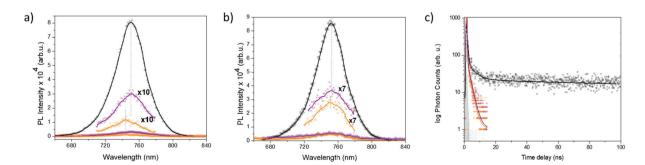
Fig. 7 Steady-state photoluminescence spectra of  $FTO/TiO_2/perovskite$  (black),  $FTO/TiO_2/perovskite/Spiro-MeOTAD$  (purple) and  $FTO/TiO_2/perovskite/D35/Spiro-MeOTAD$  (orange) devices at room temperature upon excitation at (a) 482 nm and (b) 650 nm. (c) Time-correlated single photon counting spectra under 482 nm excitation probed at 750 nm obtained at room temperature.
