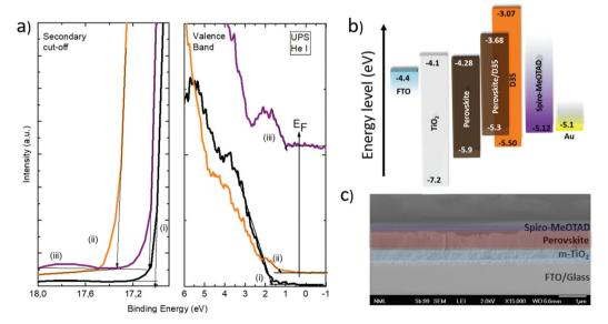
Fig. 5 UPS spectra taken from the surface of (i) ITO/TiO<sub>2</sub>/perovskite, (ii) ITO/TiO<sub>2</sub>/perovskite/D35, and (iii) ITO/TiO<sub>2</sub>/perovskite/D35/Spiro-MeOTAD samples. Secondary electron cutoff region and valence band region are depicted (a); the energy level diagram of the materials employed in the PSCs (b). A SEM cross-sectional image of a TiO<sub>2</sub>/perovskite/D35/Spiro-MeOTAD device (c).
