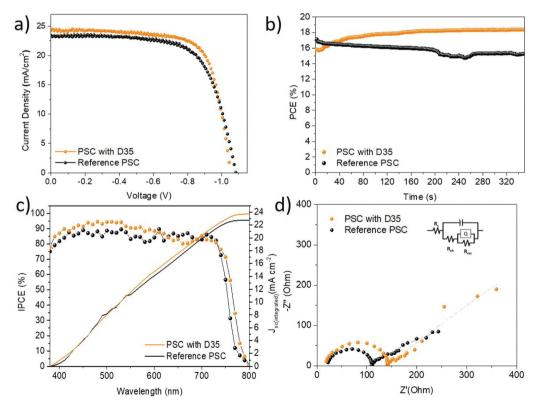
Fig. 6 The J-V curves of the best performing cells with and without D35 (a); the steady-state power conversion efficiency outputs under 1 sun illumination for reference and modified PSCs (b); the IPCE spectra and integration currents of the corresponding PSCs (c); the Nyquist plots obtained via EIS measurements, under 1 sun illumination and under  $V_{MPP}$  bias. Fitting of data is performed using the equivalent electrical circuit in the inset
