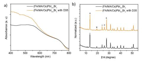
Fig. 2 UV-vis absorption spectra (a) and XRPD patterns (b) of mixed perovskite films with and without D35 treatment. Symbols "\*", "o" and "#" represent the perovskite, FTO and TiO2 peaks, respectively.
