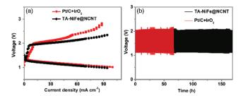
**Fig. 6** (a) Charge and discharge polarization curves of rechargeable zinc-air batteries. (b) Charge and discharge cycling curves of rechargeable zinc-air batteries at a current density of 25 mA cm<sup>-2</sup>.
