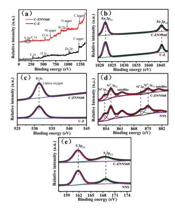
**Fig. 4** (a) XPS survey spectra of C-Z and C-ZNNS60. High-resolution XPS spectra of (b) Zn 2p, (c) O 1s of C-Z and C-ZNNS60, and (d) Ni 2p and (e) S 2p of NNS and C-ZNNS60.
