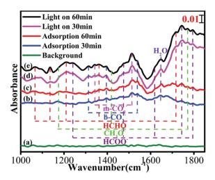
Fig. 7 In situ FTIR spectra of C-ZNNS60: (a) in the absence of CO<sub>2</sub> and H<sub>2</sub>O in the dark, after adsorption of CO<sub>2</sub> and H<sub>2</sub>O for (b) 30 min and (c) 60 min in the dark, and under light irradiation for (d) 30 min and (e) 60 min.
