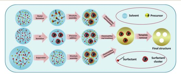
Fig. 3 Schematic representation of the general steps included in the formation of nanostructures using the soft-template: cooperative assembly, liquid crystal (LC) templating and evaporation-induced self-assembly (EISA).
