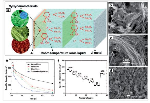
Fig. 15 (a) Schematic representation of a lithium metal battery using  $V_2O_5$  nanomaterials and room temperature ionic liquid electrolyte. SEM images of diverse morphologies of  $V_2O_5$  materials: (b) nanoribbons (c) nanowires (d) microflakes and their corresponding (e) specific capacities; (f) cycle life of  $V_2O_5$  nanoribbon. "Adapted with permission from ref. 218. Copyright (2008) American Chemical Society."
