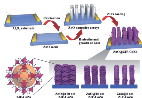
Fig. 5 Schematic illustration of the preparation of ZnO@ZIF-CoZn gas sensors. Reproduced with permission. 73 Copyright©2016 WILEY-VCH Verlag GmbH & Co. KGaA.
