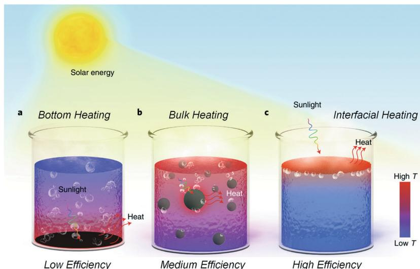
**Fig. 1** Different strategies for liquid heating using photothermal materials.<sup>10</sup> (a) Bottom heating, (b) bulk heating with suspended particles, and (c) interfacial heating with floatable substrates.
