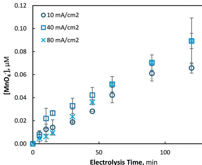
Fig. 9 Permanganate production under 10, 40 and 80 mA cm<sup>-2</sup> electrolysis conditions over 120 min (pH = 7, [Mn<sup>2+</sup>]<sub>0</sub> = 39 μM, T = 21.0 ± 0.8 °C).
