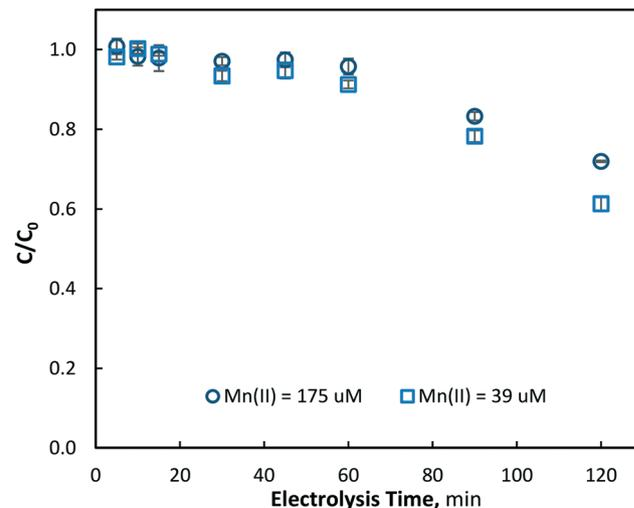
Fig. 6 Removal of aqueous manganese ( $\text{Mn}^{2+}$ ) with electrolysis time at  $40 \text{ mA cm}^{-2}$  with  $[\text{Mn}^{2+}]_0 = 175$  and  $39 \mu\text{M}$ , ( $\text{pH} = 7$ ,  $T = 21.0 \pm 0.8 \text{ }^\circ\text{C}$ ).
