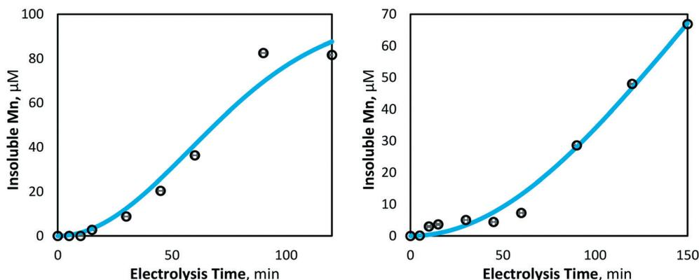
Fig. 7 Model and experimentally yielded results of insoluble manganese ( $\text{Mn}^{3+,4+}$ ) generation at  $80 \text{ mA cm}^{-2}$  (left) and  $40 \text{ mA cm}^{-2}$  (right) ( $\text{pH} = 7$ ,  $[\text{Mn}^{2+}]_0 = 175 \text{ }\mu\text{M}$ ,  $T = 21.0 \pm 0.8 \text{ }^\circ\text{C}$ ).
