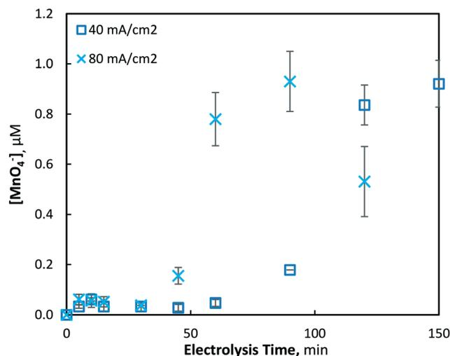
Fig. 8 Production of permanganate at  $40$  and  $80 \text{ mA cm}^{-2}$  over  $120 \text{ min}$  of electrolysis ( $\text{pH} = 7$ ,  $[\text{Mn}^{2+}]_0 = 175 \text{ }\mu\text{M}$ ,  $T = 21.0 \pm 0.8 \text{ }^\circ\text{C}$ ).
