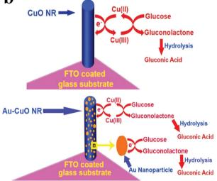
Fig. 11 (a) Schematic diagram of Au@CuO nanomaterial synthesis (b) schematic representation of the glucose sensing mechanism. Reproduced from ref. 100 with permission from Elsevier B.V., copyright 2018.
