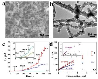
Fig. 5 (a) SEM image of  $NiCoO_2@CNT$ . (b) TEM image of  $NiCoO_2@CNT$ . (c) Amperometric responses to the successive additions of glucose. (d) The calibration curves obtained in the 0.1 M NaOH/NaAc buffer (pH 12.0). Reproduced ref. 47 with permission from Elsevier B.V., copyright 2015.
