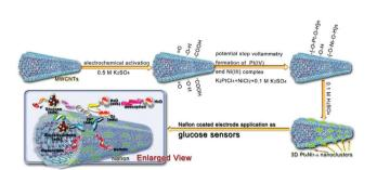
Fig. 12 Schematic diagram of the synthesis and reaction mechanism of the glucose sensor based on the flower-like 3D  $Pt_xNi_{1-x}/MWCNT$  catalysts Reproduced ref. 102 with permission from Elsevier B.V., copyright 2016.
