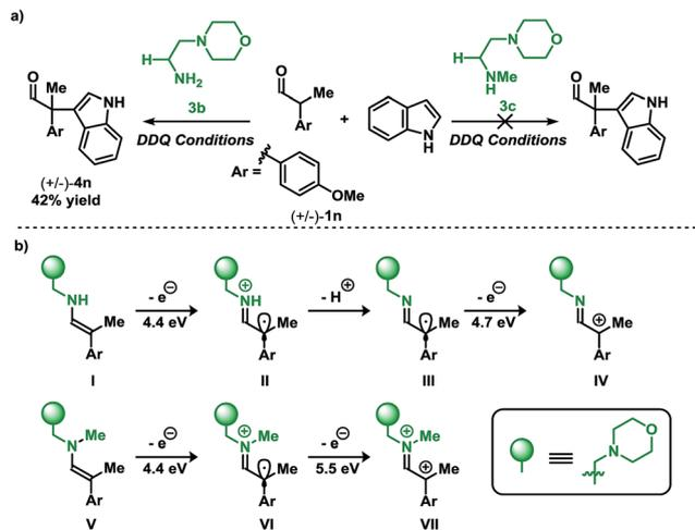
Scheme 4 (a) Organocatalyzed coupling of indoles and aldehydes: primary vs. secondary amine catalysts (see Table 2 for conditions). (b) Calculated ionization potentials for putative intermediates.<sup>12</sup>
