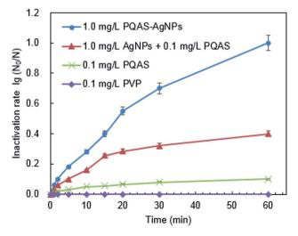
Fig. 3 The role of PQAS and AgNPs in the antibacterial activity of PQAS-AgNPs. Reaction conditions: reaction time = 60 min, pH = 7.1, T = 25 °C, initial concentration of B, subtilis:  $10^6$  CFU mL<sup>-1</sup>.
