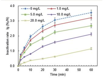
Fig. 9 Effect of HA on antibacterial efficacy to B. subtilis with PQAS-AgNPs. Reaction conditions:  $[AgNPs] = 10.0 \text{ mg L}^{-1}$ , reaction time = 60 min, pH = 7.1, T = 25 °C, initial concentration of B. subtilis:  $10^6$  CFU  $mL^{-1}$ .
