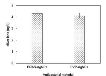
Fig. 4 The silver ion release in PQAS-AgNPs or PVP-AgNPs solution. Reaction conditions: [AgNPs] = 1.0 mg L $^{-1}$ , reaction time = 60 min, pH = 7.1, T = 25 °C.
