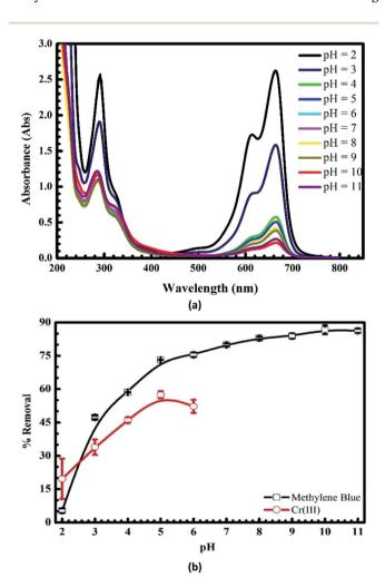
Fig. 3 UV-Vis spectra of MB after the uptake at different pH values (a) and effects of pH on the adsorption of MB and Cr(III) onto pomelo fruit peel (b).
