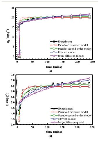
Fig. 10 Plots of kinetic models of the adsorption of MB (a) and Cr(III) (b) onto pomelo fruit peel.
