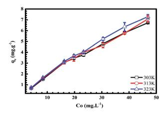
Fig. 7 Effects of initial concentration on the adsorption of  $Cr(\mbox{\tiny III})$  onto pomelo fruit peels.
