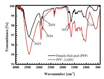
Fig. 15 FT-IR spectra of pomelo fruit peels before and after the adsorption  $Cr(\shortparallel)$ .
