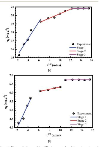
Fig. 11 Plots of intra-particle diffusion models of the adsorption of Cr(|||) (a) and MB (b) onto pomelo fruit peel.
