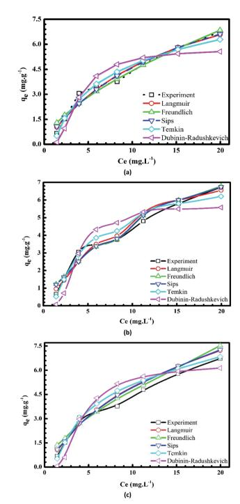
Fig. 9 Plots of nonlinear isotherm models of the adsorption of Cr(III) onto pomelo fruit peels at 303 K (a), 313 K (b) and 323 K (c).
