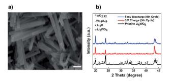
Fig. 2 (a) SEM image of an as-synthesized Li $_6$ WO $_6$  sample, the scale bar is 1  $\mu$ m. (b) XRD patterns of the as-synthesized Li $_6$ WO $_6$  (black), a sample charged to 3 V at the 5th charge cycle (red), and a sample discharged to 5 mV at the 6th discharge cycle (blue).
