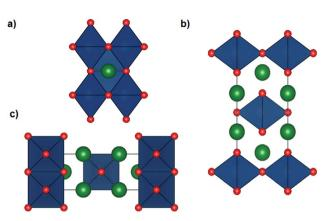
Fig. 1 Crystal structure of orthorhombic  ${\rm Li_6WO_6}$  with the space group Immm (no. 71) viewed along the (a) a axis (b) b axis and (c) c axis, where the green and red balls represent Li and O atoms respectively, and the navy blue polyhedra represent WO<sub>6</sub> octahedra accommodating a W atom (not shown) with an occupancy of 0.5.
