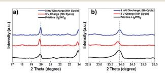
Fig. 4 Comparison of the shifts in the characteristic  $Li_6WO_6$  X-ray diffraction peaks for the as-synthesized  $Li_6WO_6$  (black) a sample charged to 3 V at the 5th charge cycle (red), and a sample discharged to 5 mV at the 6th discharge cycle (blue).
