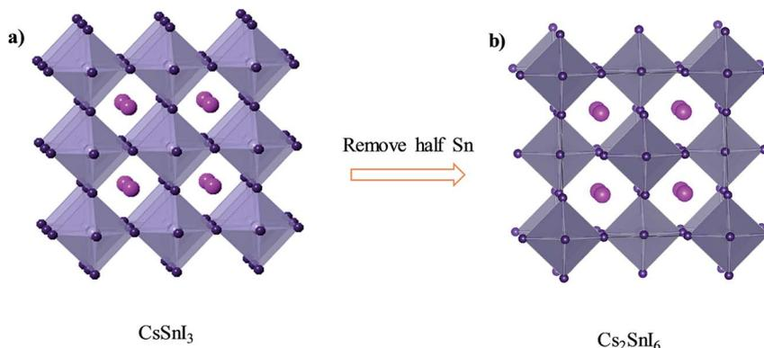
Fig. 8 (a) Crystal structure of CsSnI<sub>3</sub>. (b) Crystal structure of  $Cs_2SnI_6$ . Consulting from ref. 79.
