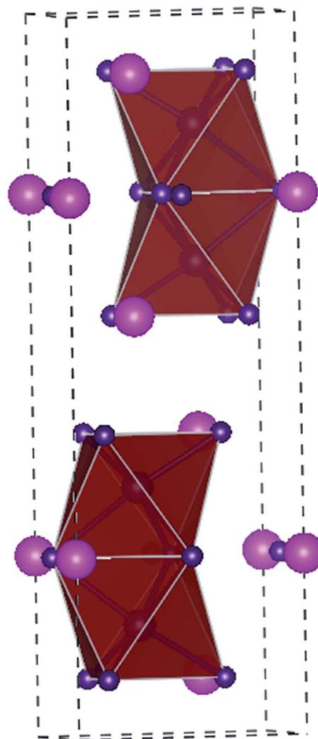
Fig. 9 Crystal structure of  $\text{A}_3\text{B}_2\text{X}_9$  perovskites. The magenta spheres represent the Cs atoms, blue spheres represent the trivalent metal atom (Bi, Sb atom), and purple spheres represent the I atom.
