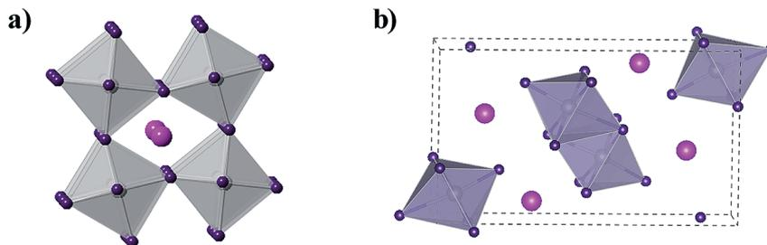
Fig. 6 (a) Crystal structure of B- $\gamma$ -CsSnI<sub>3</sub>. B(b) Crystal structure of Y-CsSnI<sub>3</sub>. In these two images, the magenta spheres represent the Cs atoms, the purple spheres represent the I atoms, and the gray spheres represent the Sn atoms.
