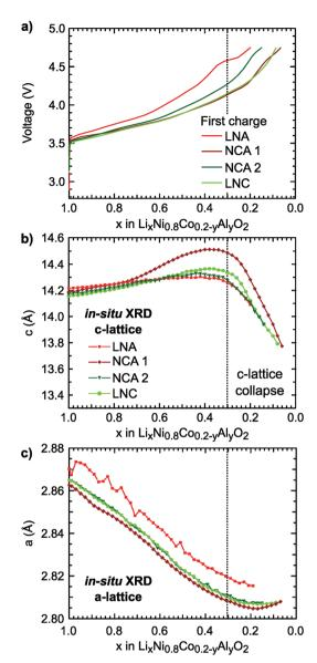
Fig. 1 (a) First charge profile for layered oxide cathodes with chemical formula LiNi<sub>0.8</sub>Co<sub>0.2-v</sub>Al<sub>v</sub>O<sub>2</sub> (0  $\leq y \leq$  0.2) to 4.75 V at 10 mA g<sup>-1</sup> (vs. Li metal) and at RT. In situ (b) c- and (c) a-lattice parameters for the first charge at C/50 to 4.75 V followed by a potentiostatic hold at 4.75 V for the Ni-rich systems. The c- and a-lattice parameters were calculated from the (003) peak and the (101) and (003) peaks, respectively.
