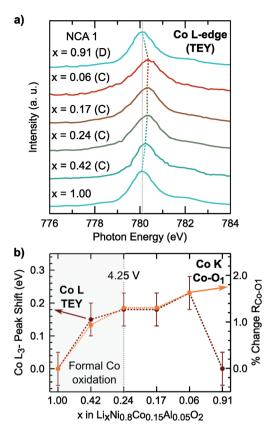
Fig. 3 (a) Co L<sub>3</sub>-edge for NCA 1 electrodes along the first charge and after full discharge to 2.7 V. The dotted line indicates the reversible shift of the main Co L<sub>3</sub>-edge peak during charge and after discharge. (b) The extent of the Co L<sub>3</sub>-edge shift is compared to the % Co-O<sub>1</sub> bond shortening extracted from EXAFS fits
