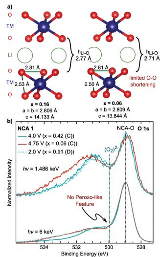
Fig. 7 (a) Nearest O-O distances based on previously reported joint XRD/ ND Rietveld refinement in the  $R\bar{3}m$  SG for NCA 1 electrodes cycled versus graphite and measured ex situ. 40 The lithium contents given here are based on the charge capacity. (b) Depth dependent XPS measurements of the O 1s core region, at 1.486 keV and 6 keV, in the formal TM redox regime (x = 0.42), after the RIXS feature onset (x = 0.06), and discharged to
