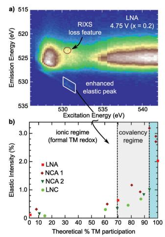
Fig. 6 (a) RIXS map of LNA electrode charged to 4.75 V (x = 0.2) showing the weak RIXS feature and corresponding enhancement of the elastic peak at 531 eV. (b) Evolution of the 531 eV elastic peak intensity compared to the expected % TM redox in the ionic viewpoint (Ni<sup>3+/4+</sup> & Co<sup>3+/4+</sup> redox couples) based on electrode delithiation and taking into account the inactive aluminum in LNA and NCA.
