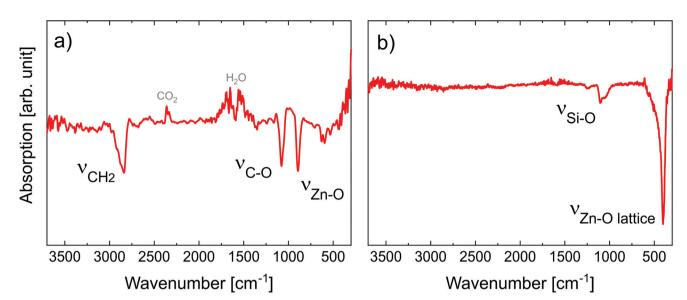
Fig. 2 FT-IR spectra of (a) 50 nm-thick MLD zincone layer right after deposition and (b) 27 nm-thick calcined MLD-derived ZnO treated up to  $600 \, ^{\circ}$ C.  $\nu$  symbols refer to the stretching modes.
