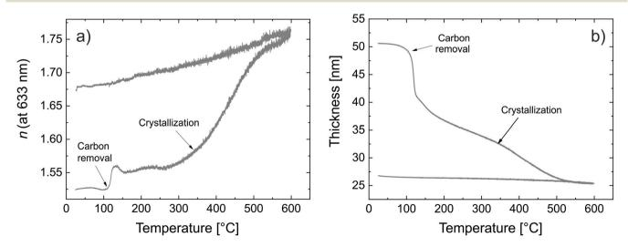
Calcination of the zincone as measured by SE (a) refractive index and (b) thickness as a function of the calcination temperature.
