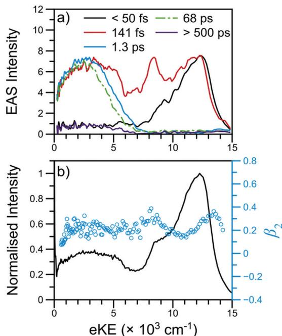
**Fig. 3** TR-PES results for NMA at 238 nm with (a) EAS and (b) the photoelectron signal (black line) and  $\beta_2$  values (blue circles) near  $\Delta t = 0$ . The short-time TR-PES transient for NMA may be found in Fig. 2; a full transient is shown in Fig. S4 of the ESI.† The EAS have been smoothed using a 3 point moving average; the  $\tau_1$  EAS intensity has been scaled for visual clarity.
