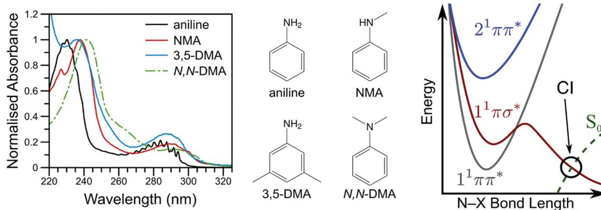
Fig. 1 The vapour phase spectra of aniline (black line), NMA (red line), 3,5-DMA (blue line), and *N,N*-DMA (green, dot-dashed line) are shown on the left with the corresponding structures shown in the middle panel. A schematic potential energy cut along the aniline N-X reaction coordinate is shown on the right (adapted from ref. 16).
