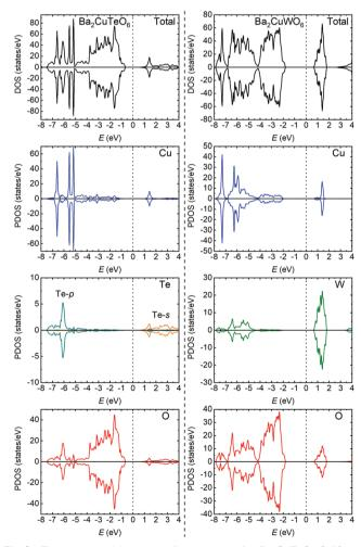
Fig. 2 Total and partial density of states plots for  $Ba_2CuTeO_6$  (left) and Ba<sub>2</sub>CuWO<sub>6</sub> (right). Both compounds are antiferromagnetic insulators. The moderate Te 5p/5s-O 2p hybridisation and stronger W 5d-O 2p hybridisation are seen in the Te/W and O PDOS plots.
