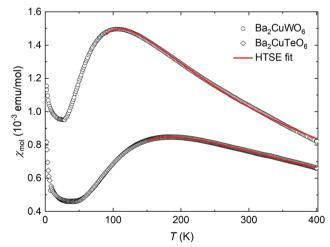
Fig. 3 Magnetic susceptibility and high-temperature series expansion fits for  $Ba_2CuTeO_6$  and  $Ba_2CuWO_6$ . Open symbols represent experimental data and the lines are HTSE fits with the parameters  $J_1 = -16.54(3)$  meV,  $J_2 = -0.04(3)$  meV, g = 2.20(1) and  $J_1 = 0.2(9)$  meV,  $J_2 = -10.0(1)$  meV, g = 2.26(5) for Ba<sub>2</sub>CuTeO<sub>6</sub> and Ba<sub>2</sub>CuWO<sub>6</sub>, respectively. The ZFC and FC curves overlap and therefore only ZFC data is shown.
