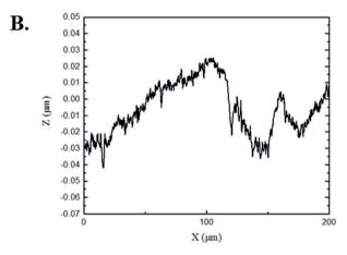
Fig. 3 3D confocal microscopy analysis of a typical experimental PDMS sample. (A) The surface shows patterns of wear which are distinct from the control visual. There appears to be some minor surface impurities. (B) Graphical height displacement across an arbitrary line on the surface.
