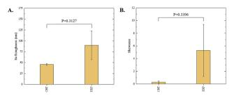
Fig. 7 Summary of (A) average  $S_a$  and (B) average  $S_{sk}$  roughness parameters of control and experimental samples *via* interferometry techniques. Error bars represent the standard error of the mean. N=5.
