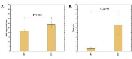
Fig. 4 Summary of (A) average  $S_{a}$  and (B) average  $S_{sk}$  roughness parameters of control and experimental samples *via* 3D confocal microscopy techniques. Error bars represent the standard error of the mean. N = 5.
