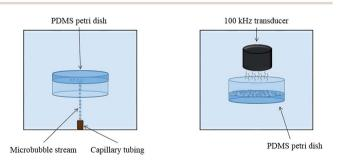
Fig. 1 Design apparatus for controlled cavitation simulation on PDMS films. MBs are initially collected on PDMS films when the Petri dish is directed downward. The Petri dish is then rotated  $180^{\circ}$  and exposed to an ultrasound transducer that induces dramatic MB oscillation, resulting in cavitation.
