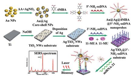
Fig. 1 Schematic of the SERS-based sandwich bioassay protocol.
