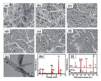
Fig. 5 SEM images of (a) TiO<sub>2</sub> NWs and Ag/TiO<sub>2</sub> NWs substrates prepared at different sputtering times: (b) 1, (c) 2, (d) 3, (e) 4, (f) 5 min; (g) TEM image of Ag/TiO<sub>2</sub> NWs; (h) EDXS spectrum of Ag/TiO<sub>2</sub> NWs substrate; (i) XRD spectra of TiO2 NWs and Ag/TiO2 NWs substrate (A, R, S, Ti and Ag represent anatase, rutile, sodium titanate, titanium and silver, respectively).
