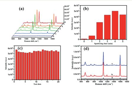
Fig. 6 (a) SERS spectra and (b) the intensities of SERS peaks at 1078 cm<sup>-1</sup> of 4MBA (10 mM) dropped on the surfaces of Aq/TiO<sub>2</sub> NWs substrates prepared at different sputtering times; (c) the intensities of the SERS peak at  $1078 \text{ cm}^{-1}$  collected from 20 random testing spots on the optimal SERS-active substrate; (d) Raman spectra of 4MBA powder on a quartz slide (line a), the freshly prepared substrate (line b) and the saved substrate (line c)
