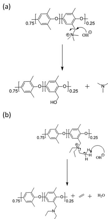
Scheme 3 (a) PPO-TMA degradation through the S<sub>N</sub>2 mechanism, and (b) PPO-TEA degradation through the E2 (Hofmann elimination) mechanism.
